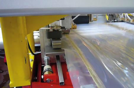
Friul Filiere has achieved important results in the agricultural sector with a complete turn-key project for the production of recyclable PE protective film. In order to make the cloth 100% recyclable, the traditional metal eyelets have been replaced with reinforced co-extruded side bands.
